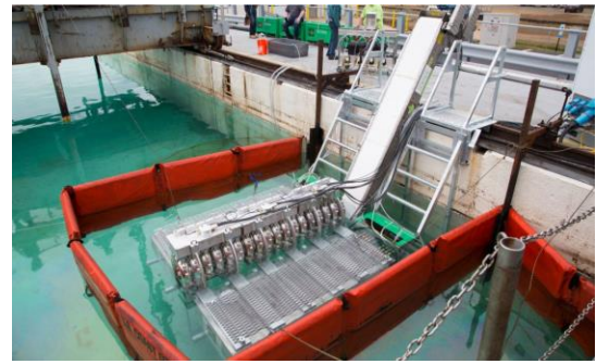
Continuous retrieval with a magnetic ramp
